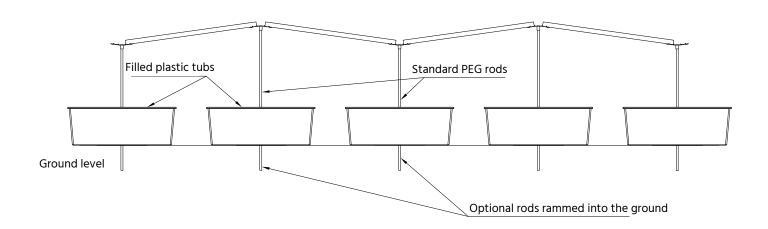
Plastic mortar tubs or high density plastic plant pots, one per rod, are filled with recycling material as a cost effective ballast solution for the PEG System. The plastic tubs are available in different shapes and sizes , eg round and rectangular, which should be evaluated based on the required amount of filled material and the required gaps between the tubs for access under the PEG for O&M activities.
