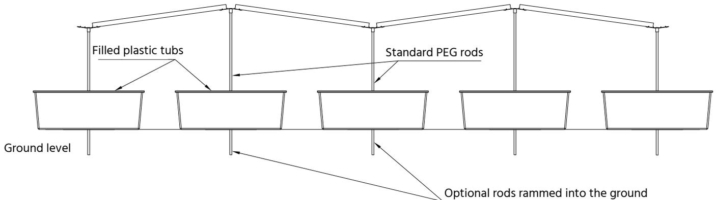
Plastic mortar tubs or high density plastic plant pots, one per rod, are filled with recycling material as a cost effective ballast solution for the PEG System. The plastic tubs are available in different shapes and sizes, eg round and rectangular, which should be evaluated based on the required amount of filled material and the required gaps between the tubs for access under the PEG for O&M activities.
